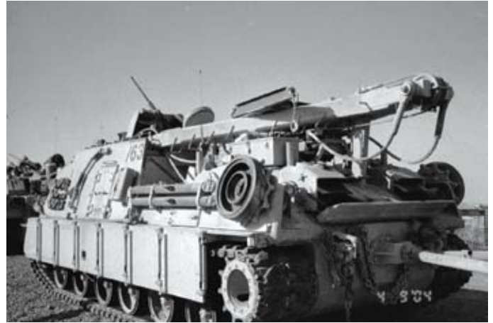
M88A2 Heavy Equipment Recovery Combat Utility Lift and Evacuation System (HERCULES)
